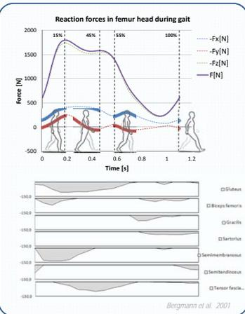
A gait cycle was simulated introducing the reaction forces and the principal muscle contributions. Tension and compression stresses were analysed in lateral and medial stem surfaces. A stress concentration peak was found in replacement stem. Also the mechanical loads transmitted to the bone were measured. While replacement stem did not transmit high loads, PROSIC one maintains a stress distribution avoiding bone resorption and stem loosening.
