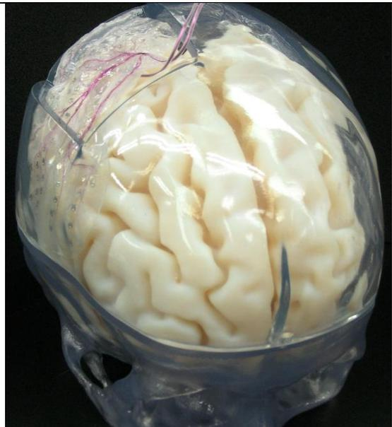
Figure 14. Inter-sulcal and Gyral surface electrodes
