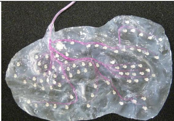
Figure 13. Single layer sub-dural electrodes for placement on the brain surface.
