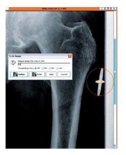
OrthoView QuickScale™ tool makes scaling the digital image quick, easy and accurate.
