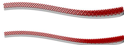
UV based conformal lattice without unit cell height preservation
