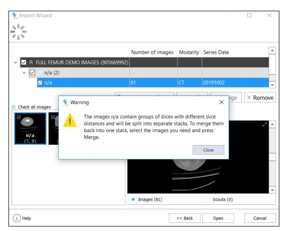
In case variability can be solved by splitting the image set in question into 3 or less image sets, the image sets are split in the New Project wizard. Image sets will never be split into more than 3 parts.
