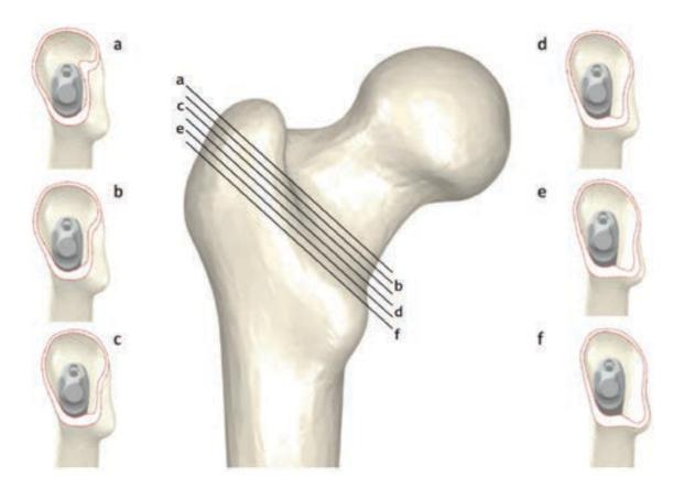
Using the model femurs, standardized cross sections were located and then used to design and verify the optimal shape for the TaperFill hip stem proximal body. Image courtesy of DJO.
